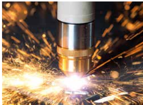
Precision Plasma cutting with automatic gas console allows Messer Hole Technology.
