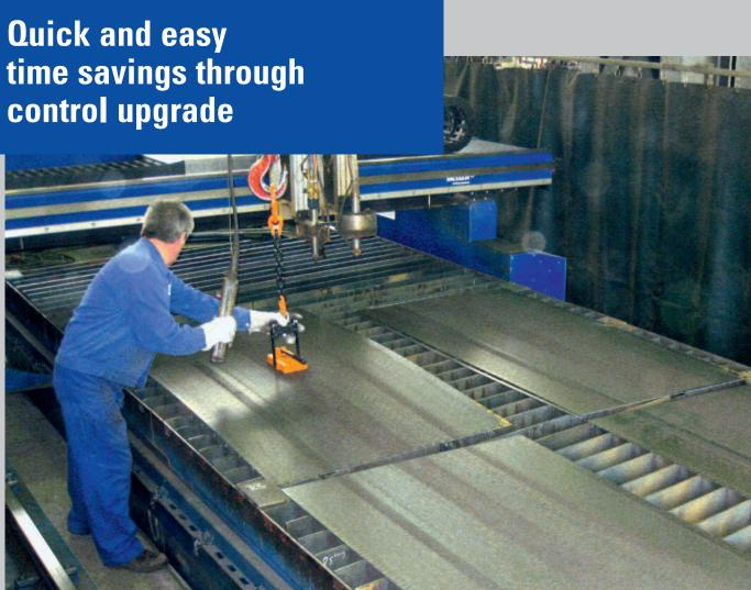
Efficient production cycles at Spinner Stahlbau GmbH: The "Joblist" function on the Messer Global Control CNC makes it possible to load four plates at a time to cut them then one after the other with the Messer MultiTherm®.
